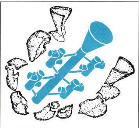
7 Mould Removal The "spent" shell is removed from the casting assembly or 'tree'.
